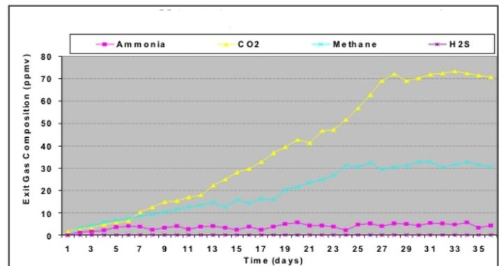
These results showed that less than 3 ppm **ZymeOut™** eliminated the formation of hydrogen sulfide, inhibited the formation of ammonia from about 25 ppmv to 5 ppmv, and increased methane production from about 24 ppmv to 31ppmv in the wastewater under anaerobic conditions
