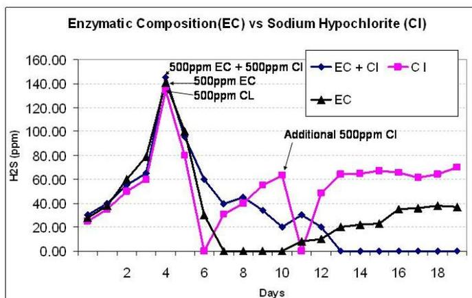
**This data shows how ZymeOut™ works to expose the bacteria that are “hiding in the slime layers” so that the biocide can be extremely effective. The hypochlorite does not work alone. Repeated doses cannot penetrate the slime layers.**
